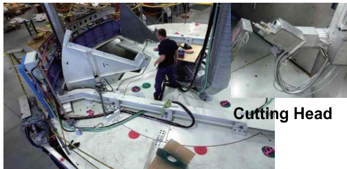
Reactor Vessel Segmentation Mock-up
